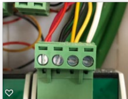
11. 13 – CAN bus with termination resistors
